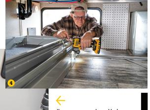
Having a cargo tray that slides both directions makes it convenient for use in an RV pass-through storage compartment. We used MORryde's 80% sliding tray (20-by-72 inches) in this application.
