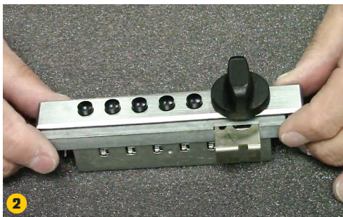
1) Lockboxes can be mounted in many locations in an RV. This one was installed in a cabinet over the cooktop. 2) The popular SIMPLEX lock is a push-button system that has five buttons and a turn knob, with 1,082 possible combinations. The buttons can be pushed individually in any order and/or multiple buttons pushed at the same time.
